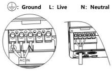
3 Properly connect the AC output wire according to the wire sequence and terminal position shown in the f below. Please connect the ground wire first, and then the live wire and the neutral wire. The ground wire is connected to the grounding screw hole on the cabinet through the O-type terminal.
