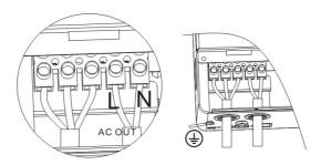
**Note:** The grounding wire shall be as thick as possible (cross-sectional area is not less than 4mm<sup>2</sup>). The grounding point shall be as close as possible to the all-in-one solar charge inverter. The shorter the grounding wire, the better.
